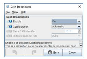
To display ethanol content, the "CAN Realtime Data Broadcasting" must be enabled. Go to "CAN bus/Testmodes menu and select "CAN Realtime Data Broadcasting". Set "Enable reatime..." to ON and set the "Base message identifier" to default value (1520). Then set a "Broadcasting rate" to 10hz.
