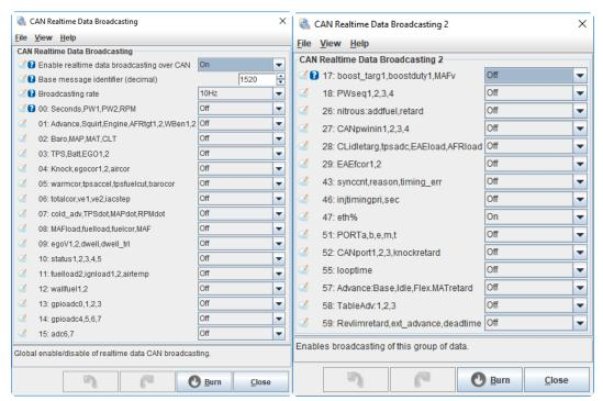
Then, click on "CAN bus/Testmodes" again and select "CAN Realtime Data Broadcasting 2". Set value "47:eth%" to ON.
